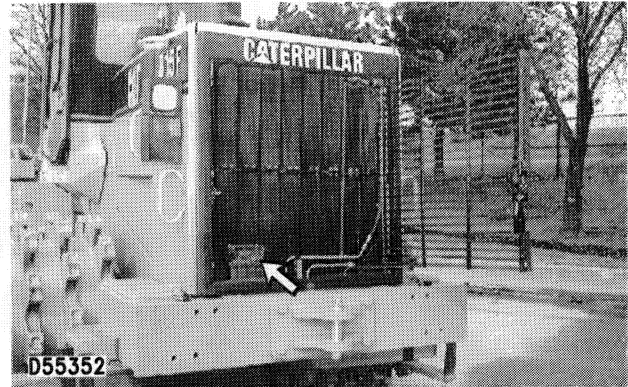
Backup Alarm – The alarm will sound when the transmission control lever is in the reverse position. It is used to alert people behind the machine that it is backing up.
